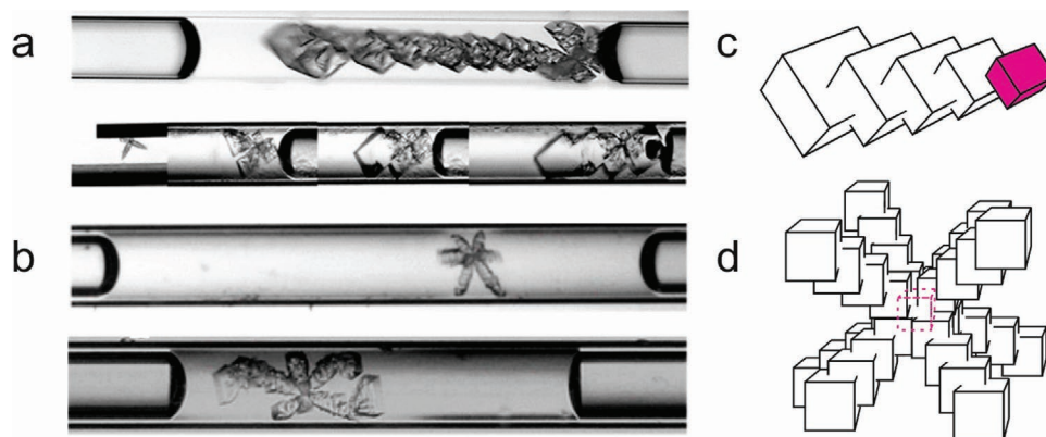
Figure 13. a) Spontaneous growth of hopper crystals at supersaturation S \approx 1.6 , in capillary of 100 \mu\text{m} (top). Evolution of the growth of a hopper crystal over 10 min (bottom). Reproduced with permission. [169] Copyright 2014, American Chemical Society. b) Multibranch hopper formed in NaCl solution with CTAB (top) and the solution with Tween 80 (bottom). c, d) Schematic of a one branch and multibranch hopper crystal, respectively. b) Reproduced with permission. [170] Copyright 2017, American Chemical Society. c, d) Adapted with permission. [170] Copyright 2017, American Chemical Society.
